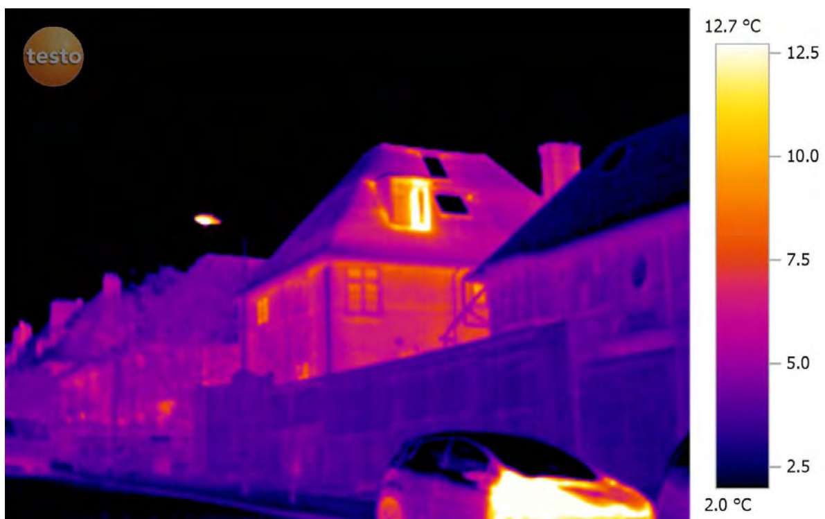
Figure 2-1. This thermal imaging picture shows significant heat leakage from a house in the same street as the Camden Passive House. Problem houses typically feature un-insulated solid brick walls, poorly insulated roofs and open windows.
